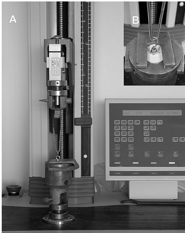
FIGURE 2. (A) Tensile test equipment. (B) Close-up view of the cast nickel-chromium bracket holder.
