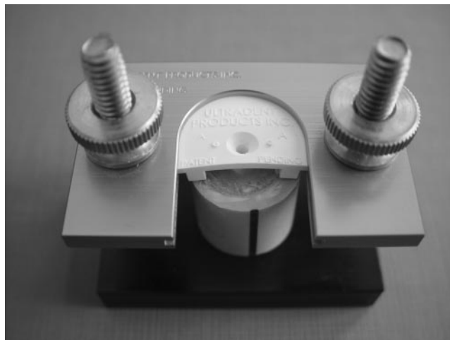
FIGURE 1. Application apparatus of orthodontic composite on the enamel surface.
