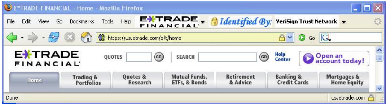
Illustration 5 An SSL protected page with TrustBar, with user-defined (or default) logo, and identification of the Certificate Authority.
