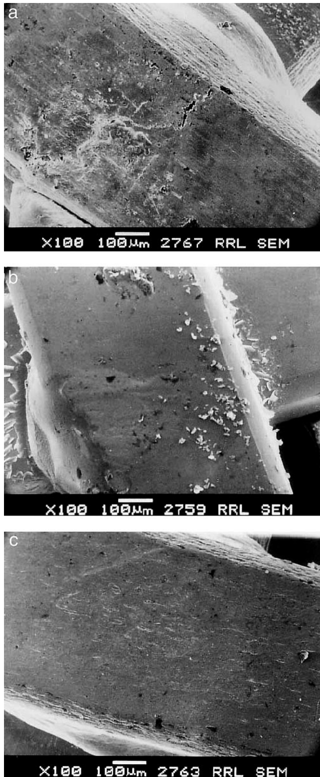
FIGURE 3. Scanning electron micrograph for surface evaluation. 100 \times magnifications. (a) Beta titanium. Note the crack propagation from point of electrode contact. (b) Stainless steel. Note peeling off of surface layer. (c) Timolium. Note smooth flow on both edges of weld area.
