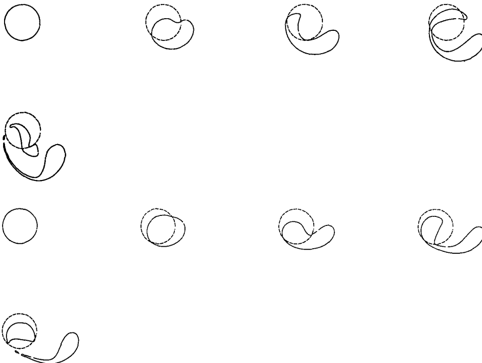
FIG. 13. Time evolution of the contour that delineates fluid that originated over the topography in the upper layer in the two-layer finite topography model for (a) \Gamma = 0.25 , \delta = 1 , and h_0/\epsilon = 2.5 at t = 0, 1, 2, 3, 4 and (b) \Gamma = 4 .
