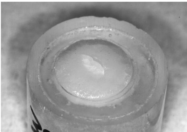
FIGURE 2. Surface destruction categorized as crack. Crack without defect can be recognized.
