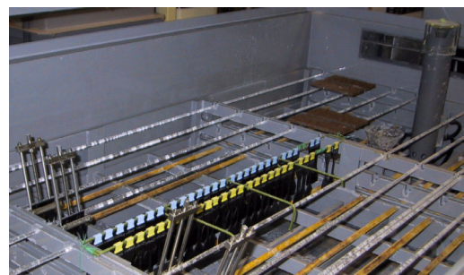
(d) Salt water and acid rain mist combined cycle test
