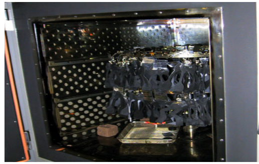
(a) Thermal oxidation test
