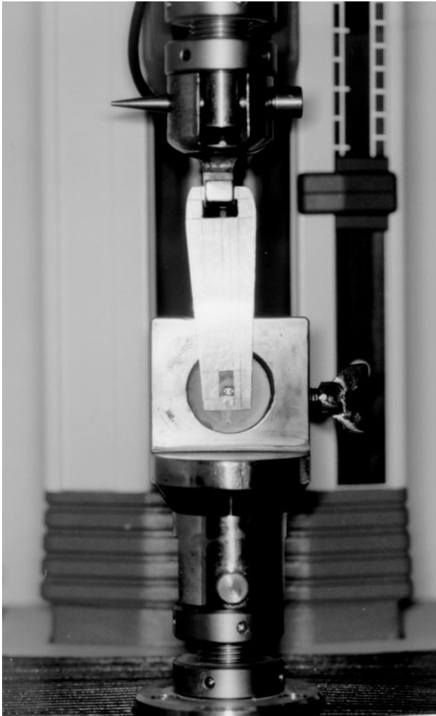
FIGURE 1. Shear test equipment used in this study.
