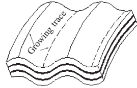
Fig.4 Model of nacre structure
