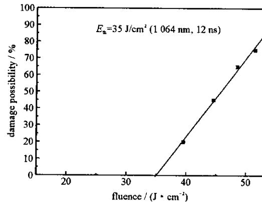
Fig. 6 Laser-induced damage threshold for the deposited sample
