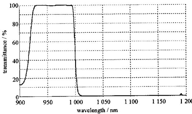
Fig. 3 Design curve for the wavelength separator with two side films on BK7 substrate
