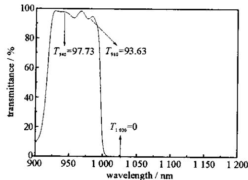
Fig. 5 Measuremental curve for the wavelength separator with two side films on BK7 substrate
