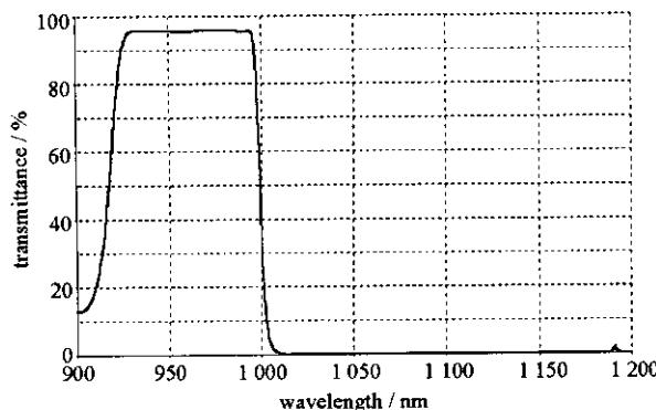
Fig. 1 Design curve for the wavelength separating multilayer
