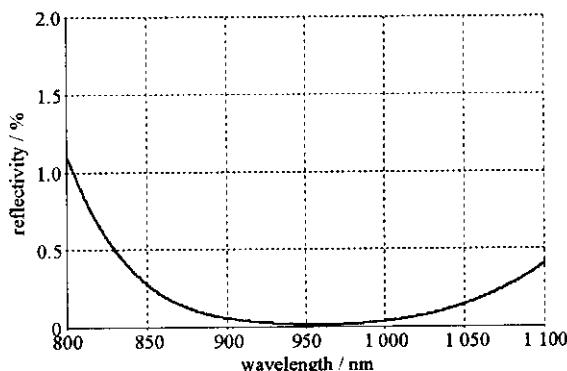
Fig. 2 Design curve for wide-band antireflection film
