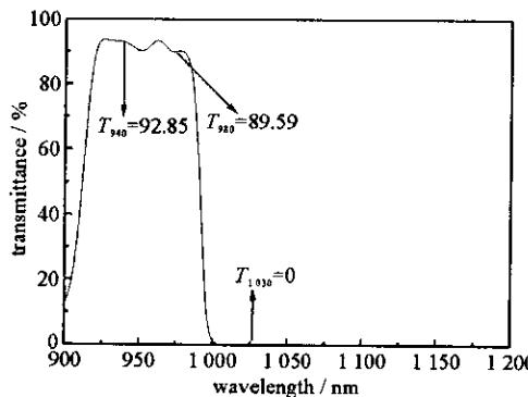
Fig. 4 Measuremental curve for the wavelength separator with one side film on BK7 substrate
