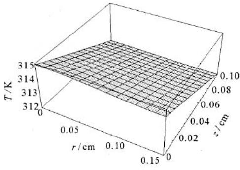
Fig. 2 Temperature rise distribution in InSb
