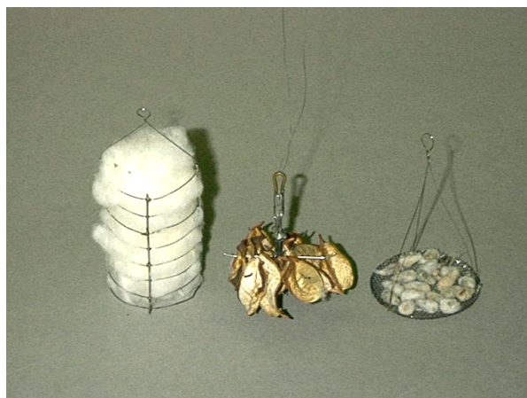
Fig. 2. Sample holders for lint, burs, and seed. Two baskets were used for lint: the smallest was 14.67 cm 2 (2.27 in 2 ) and the largest was 19.97 cm 2 (3.10 in 2 ) in cross-sectional area. The burs occupied approximately 14.45 cm 2 (2.24 in 2 ) and the seed hanger occupied 22.88 cm 2 (3.55 in 2 ).
