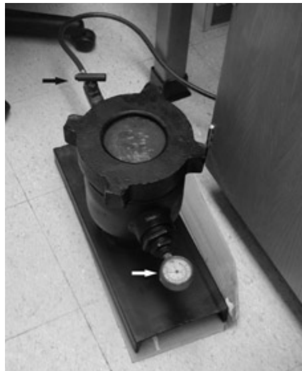
Fig. 2. Pressure chamber for nitrous oxide treatment of seedlings flanked by the chamber gas valve (black arrow) and pressure gauge (white arrow). The chamber was accessed by unscrewing the circular top (ca. 24-cm diameter).
