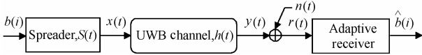
图 1 基于自适应接收机的单用户 DS-UWB 系统原理框图 Fig.1 Block diagram for a single-user DS-UWB system based on the adaptive receiver
