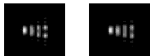
图10 R_{Tg} = 100\text{km} 时的成像结果 图11 R_{Tg} = 150\text{km} 时的成像结果 Fig.10 The image of points with R_{Tg} = 100\text{km} Fig.11 The image of points with R_{Tg} = 150\text{km}
