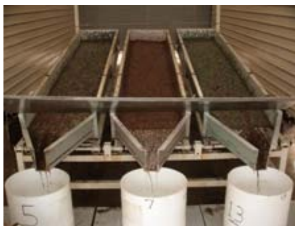
Figure 3. The erosion trays in the rain simulator.
