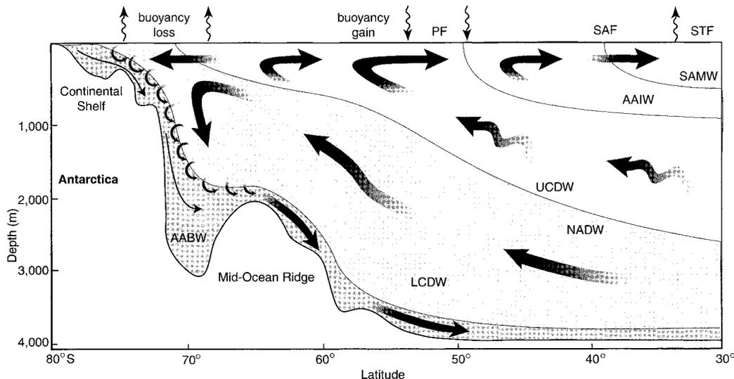
FIG. 8. Schematic two-cell meridional overturning circulation in the Southern Ocean. An upper cell is primarily formed by northward Ekman transport and southward eddy transport in the UCDW layer. A lower cell is primarily driven by dense water formation near the Antarctic continent.
