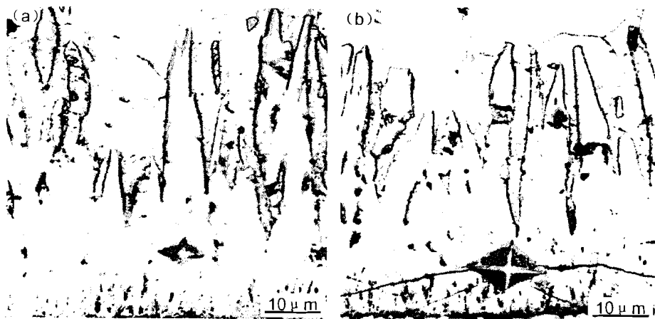
Fig.3 Micro-indentation on Fe-B compound layer (a)1# sample, (b)3# sample
