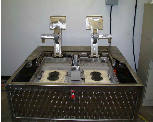
Figure 2. Hamburg wheel tracking device.
