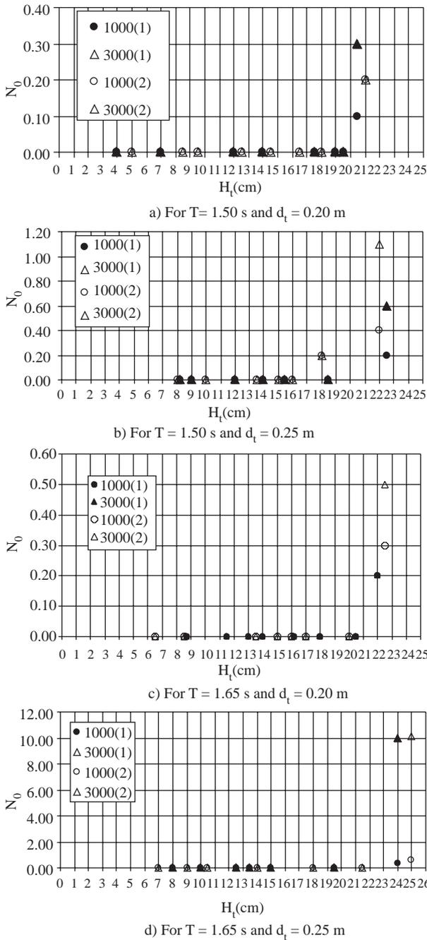
**Figure 7.** Relative damage of core-loc<sup>TM</sup> for the different wave periods and toe depths in (1) regular placement and (2) random mode.
