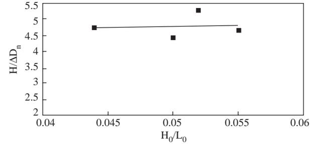
**Figure 8.** Stability number versus wave steepness for core-loc<sup>TM</sup>.
