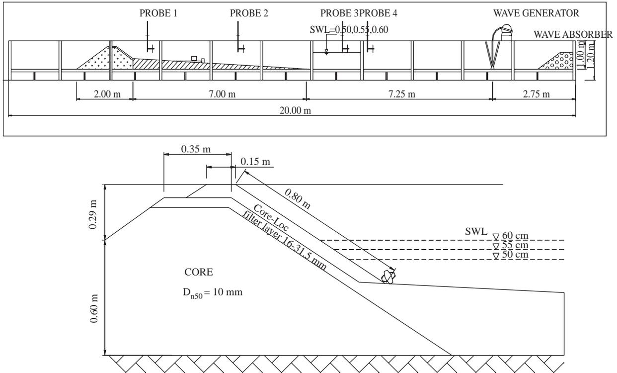
Figure 5. Experimental set-up; the wave channel and its cross section.
