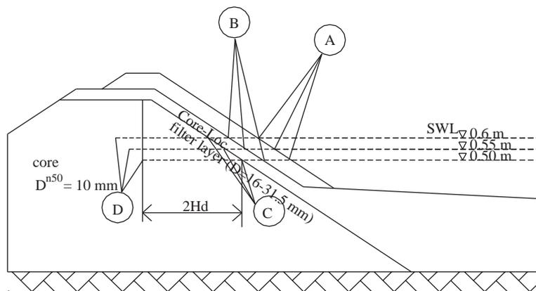
Figure 6. Run-up and run-down measurement locations in the cross section.
