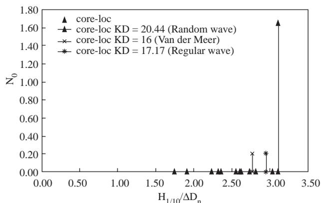
Figure 12. Stability of core-loc™ using  $H_{1/10}$ .
