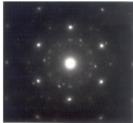
Figure 8. Electron diffraction pattern from a sample of N707 for the [111] zone axis in the T7 temper.
