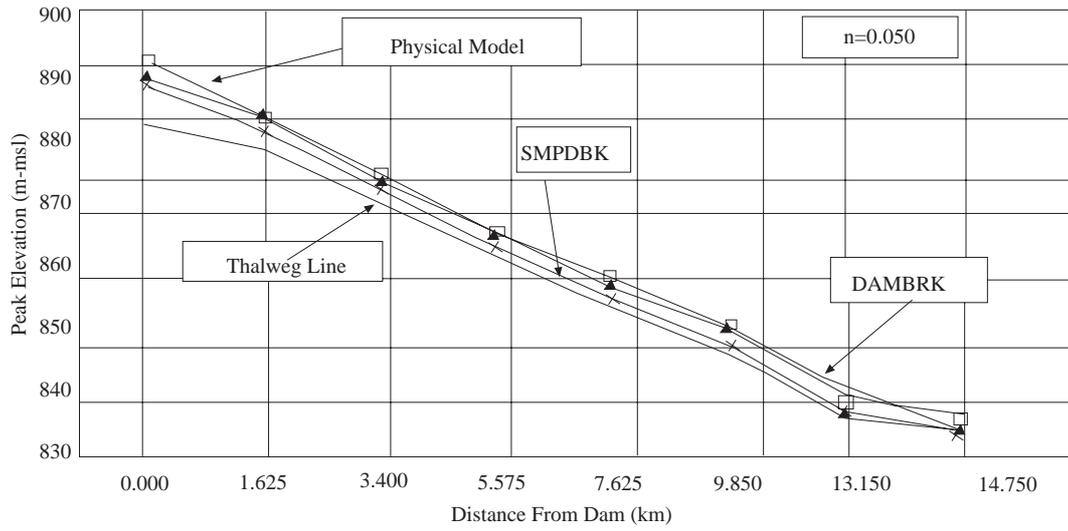
Figure 8. Peak water surface elevation vs. Distance downstream for RWSE=895.00 m.
