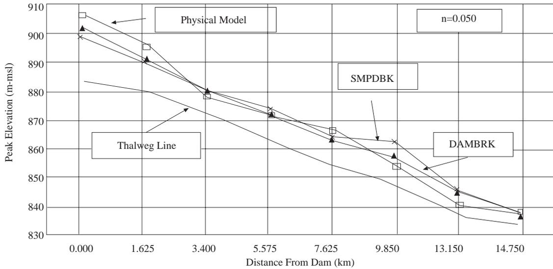
Figure 6. Peak water surface elevation vs. Distance downstream for RWSE=906.25 m.
