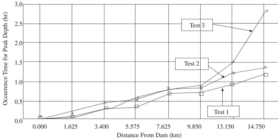
**Figure 5.** Occurrence times for peak depths at downstream stations
