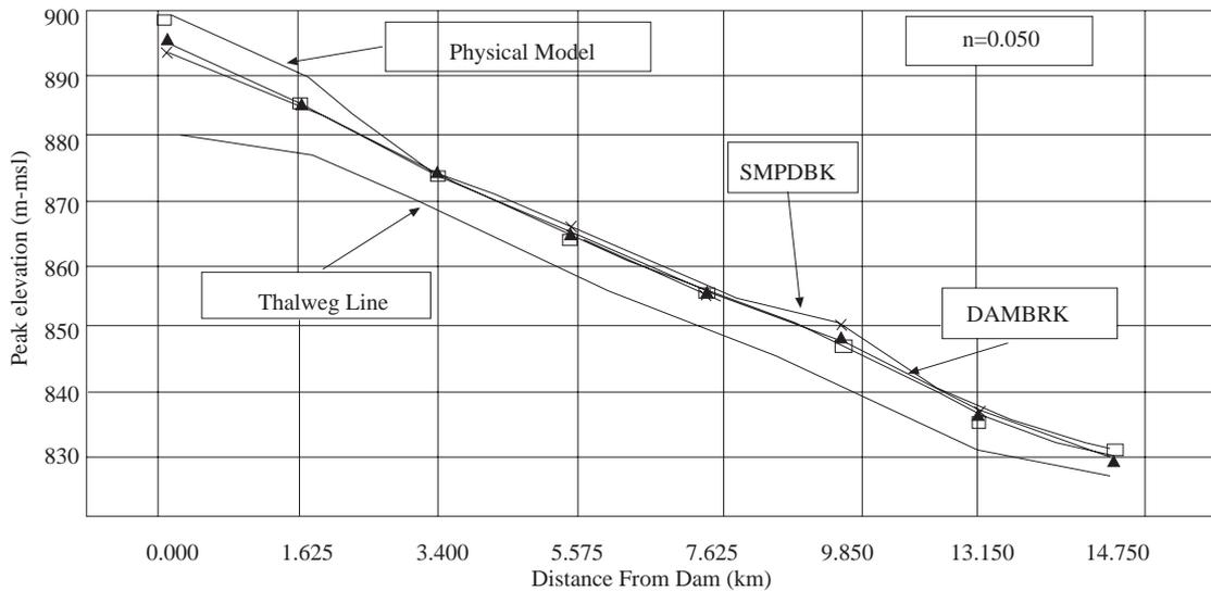
Figure 7. Peak water surface elevation vs. Distance downstream for RWSE=900.00 m.
