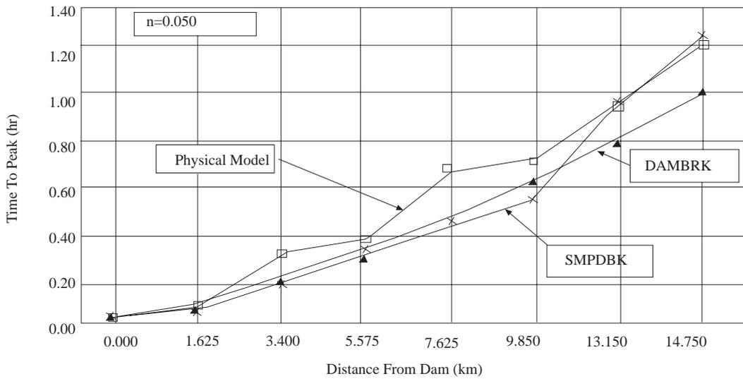
Figure 9. Peak occurrence time vs. Distance downstream for RWSE=906.25 m.
