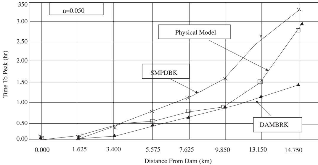
Figure 11. Peak occurrence time vs. Distance downstream for RWSE=895.00 m.
