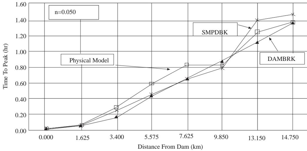
Figure 10. Peak occurrence time vs. Distance downstream for RWSE=900.00 m.
