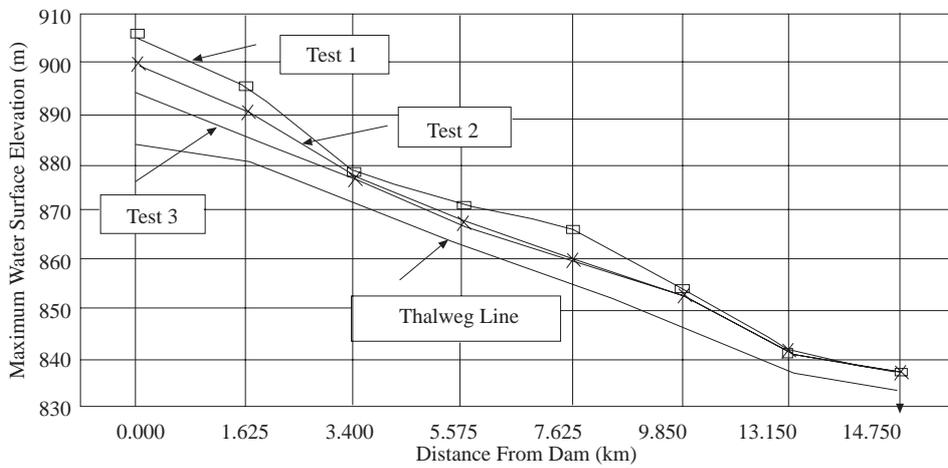
Figure 4. Peak water surface elevations measured at downstream stations
