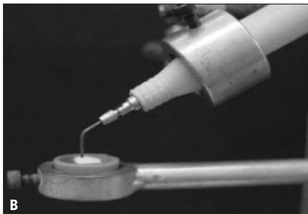
Figure 2 - Standard device for dental cavity preparation (A). CVDentus system on ultrasound device making the cavity on the specimen (B).
