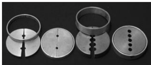
Figure 1 - Mountable metallic matrices used in the study. On the left side is the 6 mm x 4 mm matrix, dismounted and mounted, and on the right side is the 12 mm x 6 mm matrix, dismounted and mounted.
