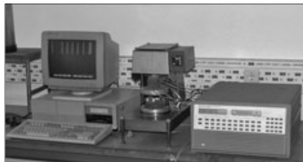
Figure 3. Measuring equipment for experimental determination of the heat transfer coefficient
