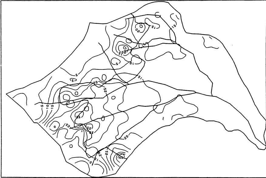
Fig. 5. Distribution of snow water equivalence in cm on Marmot Creek Experimental Basin for an average month of February, as computed from the extrapolated pin measurements.
