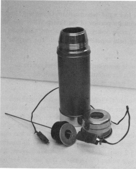
Fig. 2. Calorimeter bottle with temperature probe and rubber stopper.
