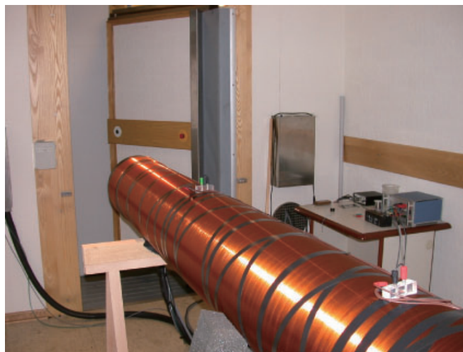
Figure 1. The great solenoid in the shielded room.
