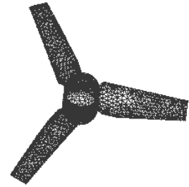
(c) Meshing for the impeller
