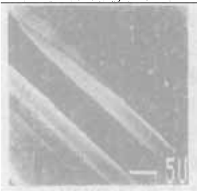
图3 未经热处理的纤维表面形貌 Fig. 3 The surface appearance of fibre before heat treatment
