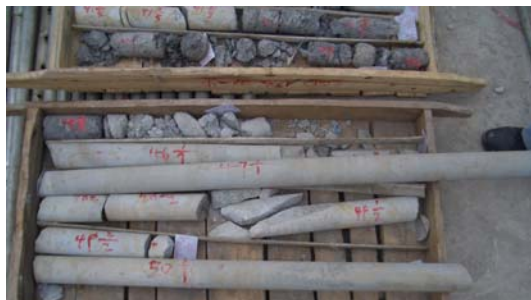
图 3 GZK01 观测孔的挤压带照片 Fig.3 Photo of fracture zone of rock core in measured borehole GZK01
