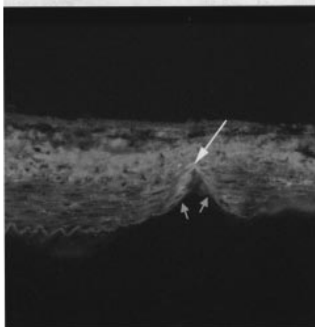
Figure 8 —Cross-sectional optical micrographs of microprobe transection through the internal elastic lamina and media in a diseased vessel by 140- \mu\text{m} -high microprobes applied with a pressure of 500 mmHg. (Top) Arrow indicates the location of microprobe application. The plaque is visible as large red areas. (Bottom) Fluorescence image shows the internal elastic lamina transected by the microprobe (two small arrows) and penetration through the media almost to the external elastic lamina.
