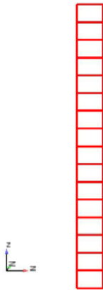
Figure 2: The one-column-cell ‘HCCI’ mesh at BDC.
