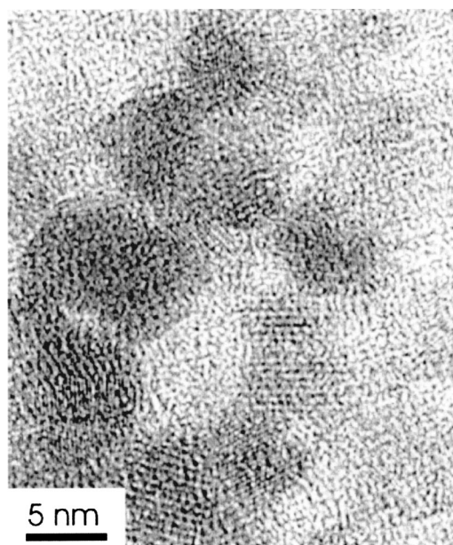
FIG. 2. TEM of NZFO nanoparticles.
