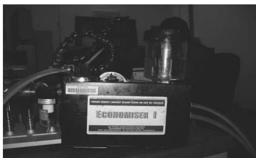
Fig. 1. MQL unit used in High Speed Milling
