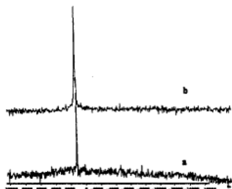
图 1 溶胶体系的 ^{14}\text{N} NMR 谱 Fig.1 ^{14}\text{N} NMR spectra of the synthetic gel mixed in \text{Na}_2\text{O}-(\text{CTMA})_2\text{O}-\text{SiO}_2-\text{H}_2\text{O} system (a) 25 °C, (b) 90 °C
