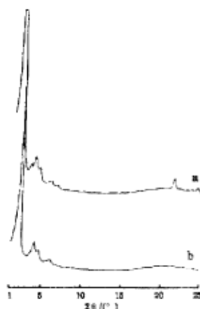
图 3 TMAOH- \text{SiO}_2 -CTMABr- \text{H}_2\text{O} 体系中不同晶化时间合成样品的 XRD 谱图 Fig.3 XRD patterns of samples synthesized in the TMAOH- \text{SiO}_2 -CTMABr- \text{H}_2\text{O} system with different crystallization time (a) 3h, (b) 5h
