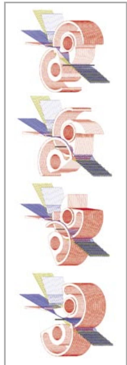
Figure 3. Succeeding positions of the elements of the mechanism which forms the shed and beating-up the warp.
