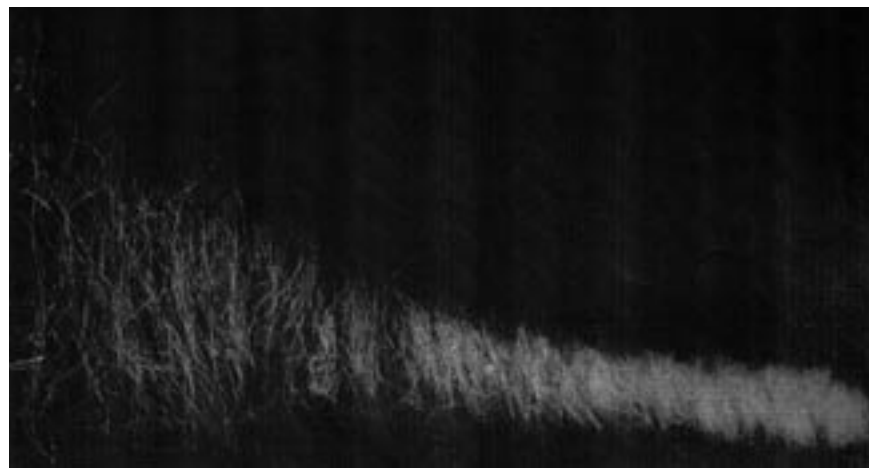
Figure 1. Distribution of fibres in the cottonised flax, mean fibre length – 27.4 mm, fibre linear density – 1.1 tex.
