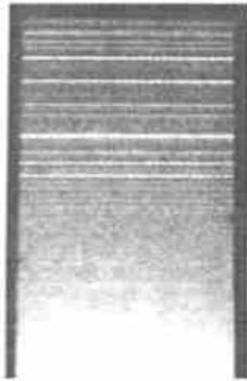
Fig. 6 Typical image of Al X-ray emission measured with 2 400 lp/mm flat-field grating spectrometer 图 6 2 400 线每毫米的平场光栅谱仪测量的时间分辨铝等离子体发射谱线典型图像
