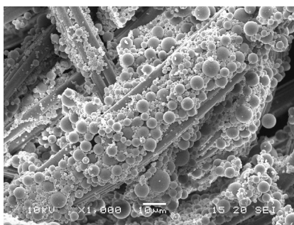
Figure 10. SEM image of nonwoven with micro-spheres (variant I – half a year storing at RH 33%).
