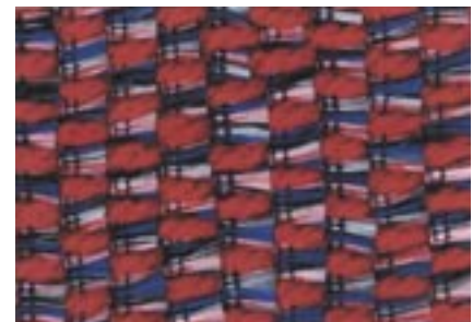
Figure 7. View of a real woven structure formed from linear haberdashery wastes as warp with the use of a multi-shed rotary loom.
