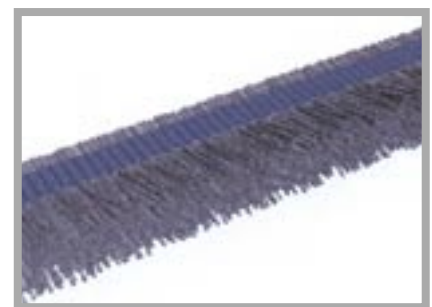
Figure 11. Virtual model of an auxiliary selvage obtained from Picanol loom.
