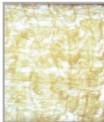
Figure 14. Real view in transmitted light of a both-side laminated composite, half-transparent, and reinforced by a woven fabric with warp from auxiliary selvages.
