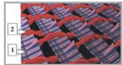
Figure 6. Virtual model for forming a woven fabric from haberdashery wastes; 1 – warp of waste, 2 – weft of yarn.
