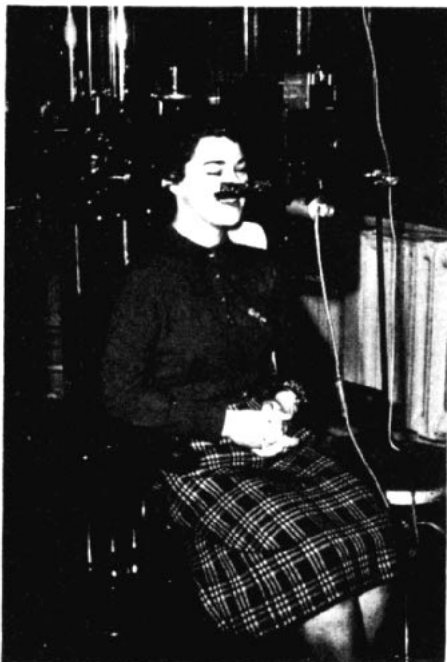
Fig. 2 Subject positioned by calibrated ear-rods and orbitale markers. The high-fidelity Altec 660B microphone is mounted exactly six inches from the lips at rest.
