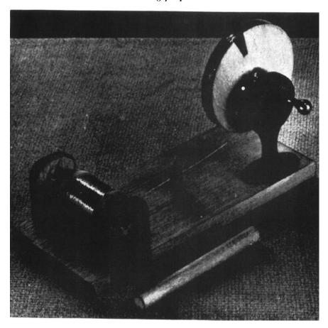
The wheel is cemented on a geared 16 mm. film rewind. This mechanism is then mounted on a wood base 5 inches by 14 inches. At the other end of the base 2 standards are placed having holes 5% and 3% inches in diameter containing wooden spindles. The different size spindles are for variations in the size of the spools.
