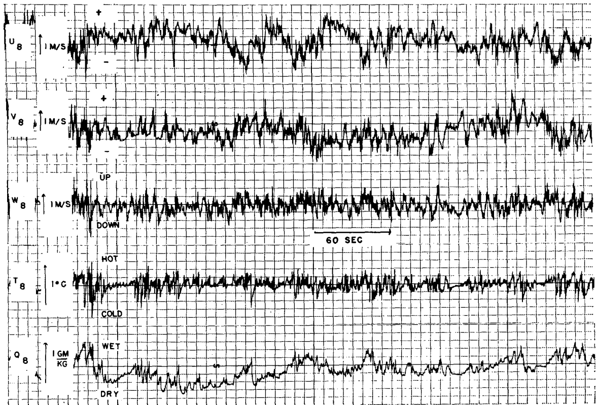
FIG. 6. Traces of u , v , w , T and q from 8 m, run 142. These data are concurrent with those shown in Fig. 5.
