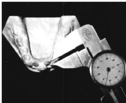
Fig. 1 Special dial caliper used to measure linear displacement of anatomic contact points.
