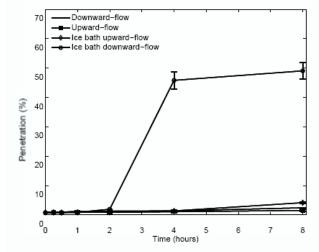
Figure 5: Experimental Results of E5 specimen exposure to ethyl benzene.
