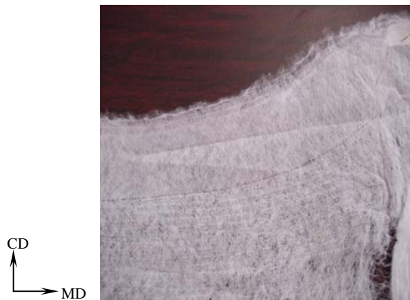
FIGURE 2. Fabric damage as a result of separating the fabric from the forming belt
