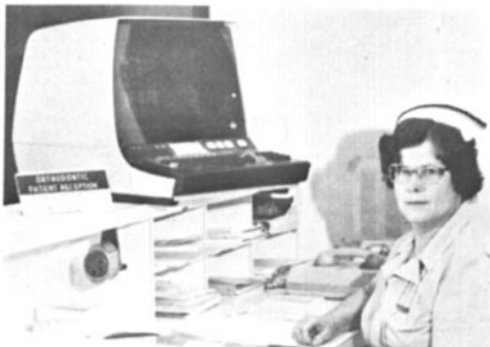
Fig. 2 Administrative records of patients are updated through a television-type terminal (Vucom) located at the reception area.
