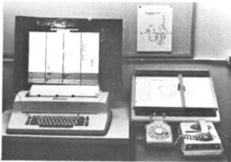
Fig. 4 An IBM 2741 terminal is used for programming and on-line plotting.
