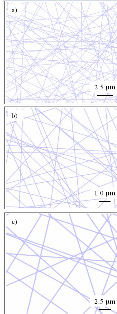
FIGURE 6. Top view of three virtual webs made of fibers with a diameter of 50, 100, and 200 nanometers, respectively. Note that the size of the scale bar is different in (a) and (c).
