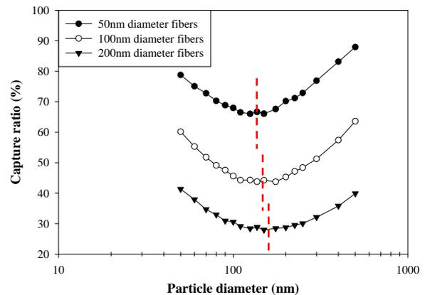
FIGURE 7. Collection efficiency of filter media made of fibers of 50, 100, and 200 nanometers diameters. All the three webs have identical thickness and pressure drops but different SVFs.
