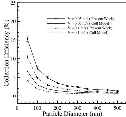
FIGURE 5. Collection efficiency vs. particle diameter [9].
