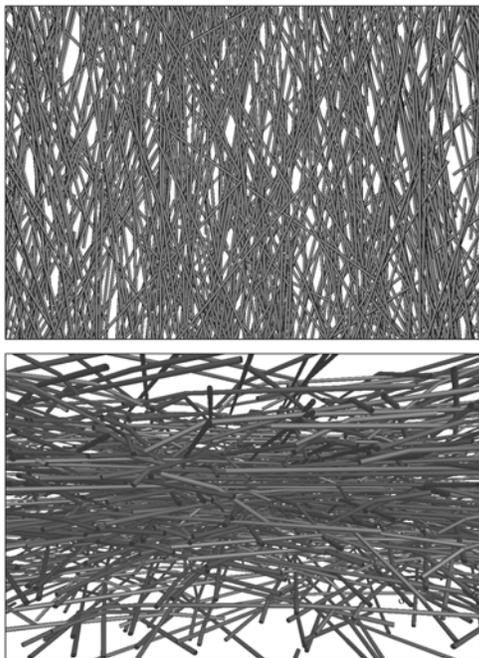
FIGURE 2. A 3-D fibrous structure generated by sequentially depositing horizontal fibers from top and side views.
