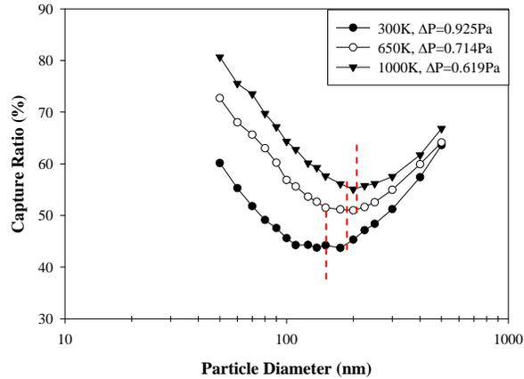
FIGURE 8. Influence of gas temperature on nanoparticle collection efficiency.
