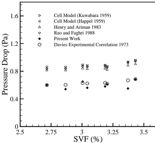
FIGURE 4. Pressure drop of our modeled microstructure in comparison with existing 2-D models. A good agreement with empirical data is evident [9].
