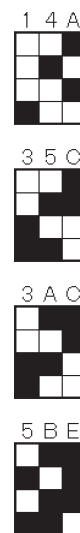
Fig. 15 Four peg plan diagrams each of which has only two equivalent diagrams.
